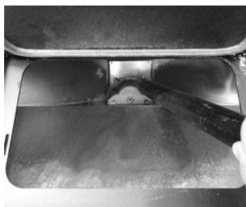
Fig. 35 - Hopper and auger cleaning
