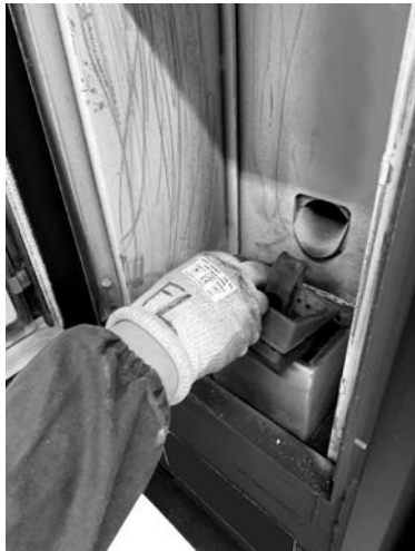
Fig. 27 - Burning pot extraction
