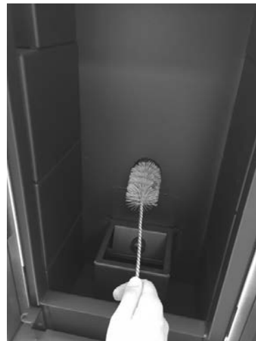
Fig. 30 - Cleaning with a brush
