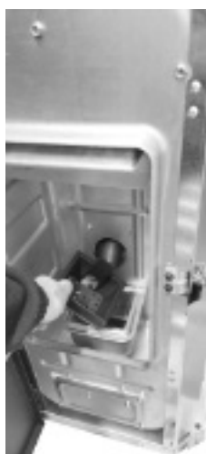
Fig. 37 - Burning pot extraction
