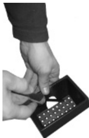
Fig. 38 - Burning pot cleaning
