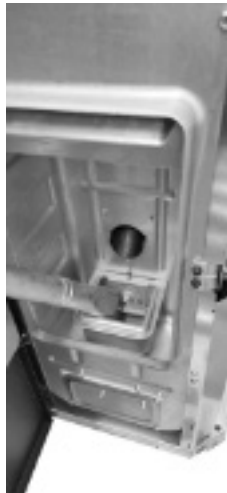
Fig. 39 - Burning pot box cleaning
