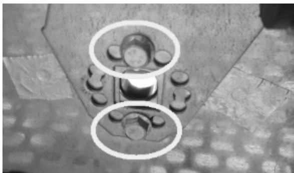
Fig. 63 - Remove the screws
