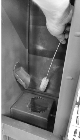
Fig. 58 - Clean with pipe cleaner
