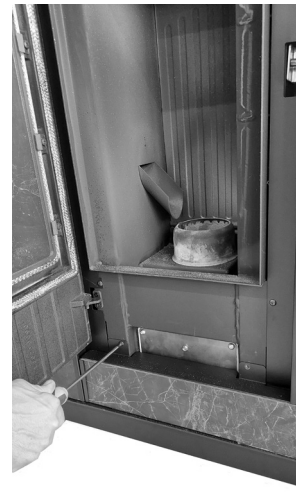
Fig. 50 - Remove the ARCO Mask
