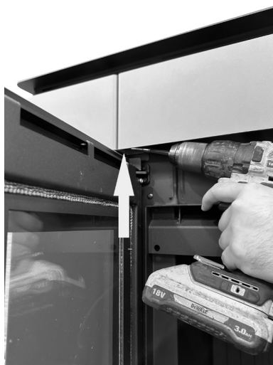
Fig. 21 - Remove the security screw
