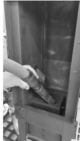
Fig. 48 - Vacuum out the ash
