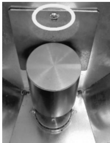
Fig. 64 - Remove the screw
