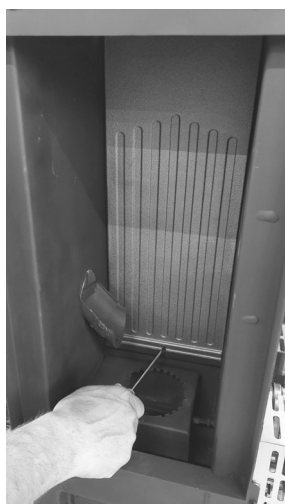
Fig. 56 - Remove the back of the hearth 1
