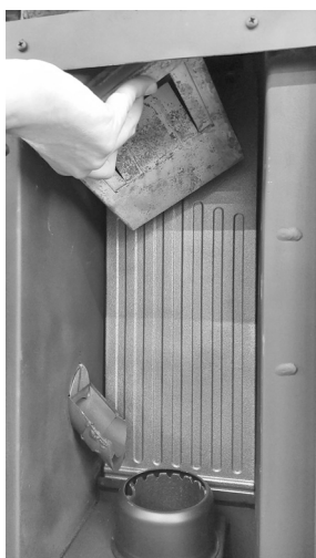
Fig. 55 - Remove the hearth head 1
