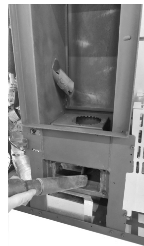
Fig. 53 - Vacuum out the ash
