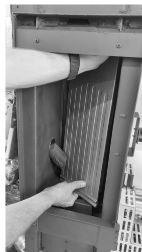
Fig. 57 - Remove the back of the hearth 2
